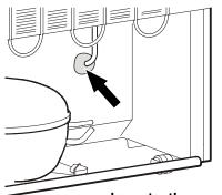
Important!4. Close the sensor cable opening at the back of the appliance with the sealant provided.
